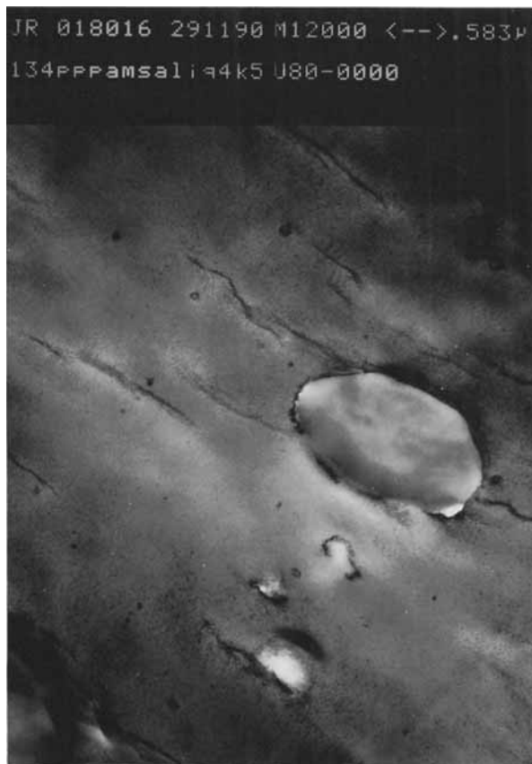
Figure 1 TEM image of PP/PA-12 (70 : 30) strained to 50% elongation.
